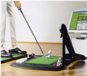
■ The Golf Achiever scans the ball, club shaft and club head. The data is then fed into a PC and analyzed.
